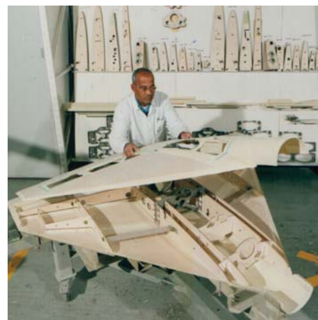
Harpy Loitering Attack UAV Composite Fuselage Construction
