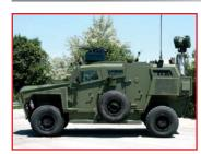
**Xtream** - A 16 Ton all terrain 4X4 MRAP, up to 7 people, KE Stanag 2 and Mine protection Stanag 3a+2b
