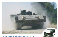
ACHZARIT-X3A-1-2 IDF "Achzarit" Heavy APC With new Power Pack, DDC 8V92T(N) 710 HP engine, and Allison XTG411-5(N) transmission.
