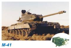
M-41/M-42 Upgrading & Modernization program with new diesel Power unit, Allison CD-500 transmission, DDC 8V71T / 8V92T engine, and new 90mm Gun/Air defence turret electronic control.
