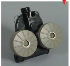
A compact and reliable air-supply unit that maintains positive pressure in military and civilian NBC protective hood systems and masks. Developed by the Israeli MOD, the blower draws filtered air from 2 standard personal NBC filters, and supplies up to 90 liter/min. Fits all types of personal filter canisters with a standard (40mm / 1/7") thread. Flat design, allowing access to narrow spaces. Special features for mounting the blower on a waist belt.
