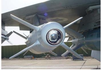
It is a new generation stand-off Precision Guided Munition (PGM). SPICE-250 has a standoff range of 100 kilometers. The SPICE-250 is an autonomous weapon with real-time target position update capability. SPICE-250 is a unitary munition and can be equipped with either general purpose or penetration warheads. The aircraft's increased load-out and wide target set provide the optimal solution for high volume precise strike for the dynamic battlefield.
