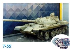
T-55 Upgrading with new Power Pack, upgraded, western gun and new fire control system.
