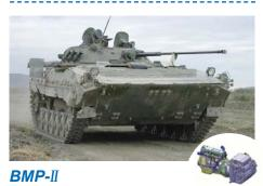
BMP-II APC Upgrading program with Western new Power Pack, Allison X-200 Transmission, and 360 HP Engine. Wide range of engines are optional.
