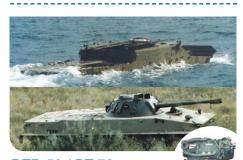
BTR-50 / PT-76 The BTR-2000 / PT-76-2000 is Nimda upgrade of the old BTR-50 / PT-76 including new engine, new gun, F.C.S, Etc.
