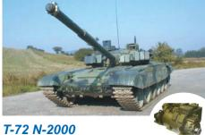
Manufacturing Allison transmission model XTG 411 6N 1000 HP Rating, For T-72 and M107/109 SPG.
