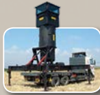
Mantis Multipurpose, self-rising, mobile, B.P. high elevated autonomous combat post
