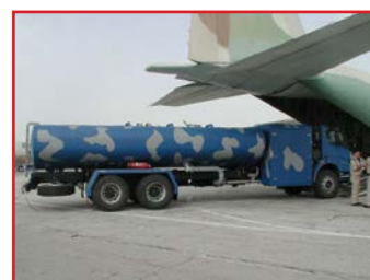
Refuellers & Tankers – Tailor made Aircraft refuellers and tankers with capacities ranging from 3000Lt-60000Lt, designed as 6X6, 6X4, 4X4 or 4X2 on/off road vehicle, can be fitted for aerial transportation
