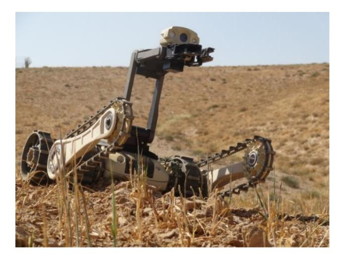
The MTGR<sup>®</sup> (Micro Tactical Ground Robot) platform is a unique and robust lightweight, man portable, tactical unmanned vehicle with high maneuverability in all terrains both indoors and outdoors with 4 DOF manipulator. Designed for ISR, EOD, and IED at urban and open terrain.
