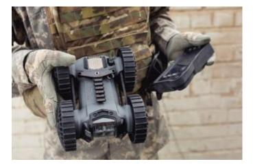
Using cameras and the microphone, suited for day and night operations, the IRIS operators are able to quickly access the hazards of dangerous situations from a safe distance, allowing the IRIS to be our first line of defense ahead of human or canine forces. The IRIS can carry a verity of add-ones for different missions. The hand-carried system is controlled by the Ruggedized Operator Control Unit (the ROCU) – a high resolution, handheld, touch-screen operator console with gamepad controllers.
