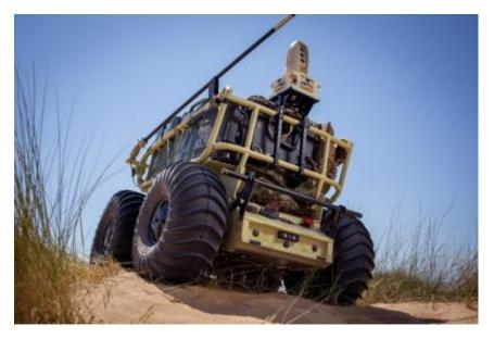
The PROBOT<sup>®</sup> (Professional Robot) is the only tactical multipurpose platform for urban terrain and outdoor operations. Its unique abilities include carrying heavy payloads while maintaining high speeds, sound maneuverability over various obstacles and performing semi-autonomous missions.
