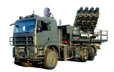
Family of Short and Medium Range Air Defense systems using the i-Derby and Python-5 missiles. designed to engage and destroy a wide spectrum of threats, such as attack aircraft bombers, cruise missiles, UAVs, UCAVs' stand-off weapons and precision guided munitions.
