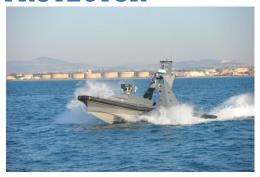
The Protector is an integrated naval combat system with anti-terror mission module payload including sensors and weapon systems, based on unmanned, autonomous, remotely controlled surface vehicles. Highly maneuverable and stealthy, the Protector can conduct a wide spectrum of critical missions, without exposing personnel and capital assets to unnecessary risk.
